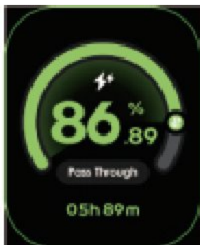
IN + OUT (Bypass on)
